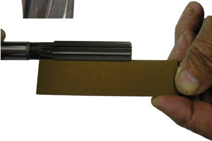
Reamers are like drills, if you use them repeatedly in aluminum they develop build-ups on the cutting edges. These build-ups effectively make the reamer larger, causing a larger hole. This larger hole then robs the bushing you're installing of interference needed to properly crush the bushing. This causes the pin to be loose in the bushing, which defeats the entire purpose. To prevent this, you need to (1) keep your reamers sharp and (2) use plenty of CUTTING OIL when reaming.
