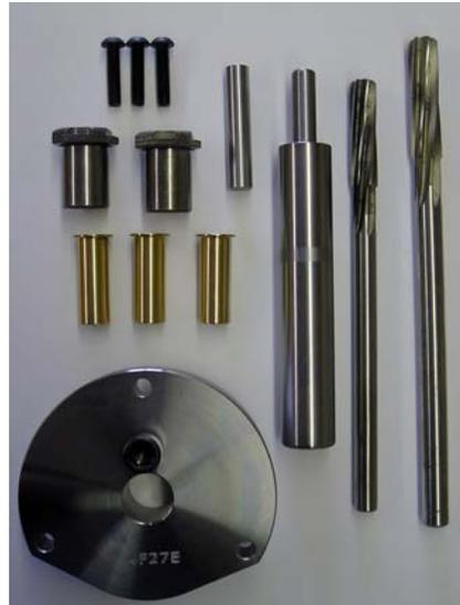
This tool is for use on **Ford 4F27E (FN4A-EL)** transaxles.
