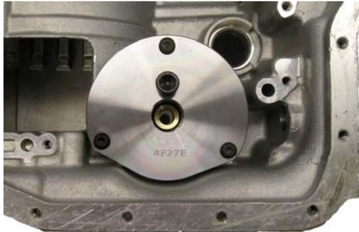
1. Install the drill jig into the case by setting the jig into the servo. Install the included 6mm bolts in the case, through the jig.
