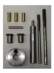
This tool is for use on Aisin TF-80SC and TF-81SC (AF20, AF21) transaxles.
