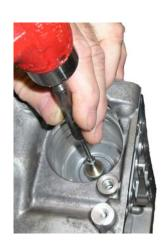
8. Insert the provided sizing pin into the bore, chamfer first. It may be necessary to start the pin in the bushing with a rubber mallet. Once the pin is inside the bushing, use a punch to drive the pin all the way through the bushing. The included sizing pin is larger than the factory servo pin, so repeat until the factory servo pin moves freely through the bushing.
