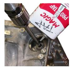
7. Apply Loctite® (preferably green #680) or equivalent to the bushing and drive the bushing in by hitting the driver until the bushing bottoms.
