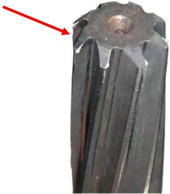
Inspect for aluminum buildups on the cutting edges as pictured left.
