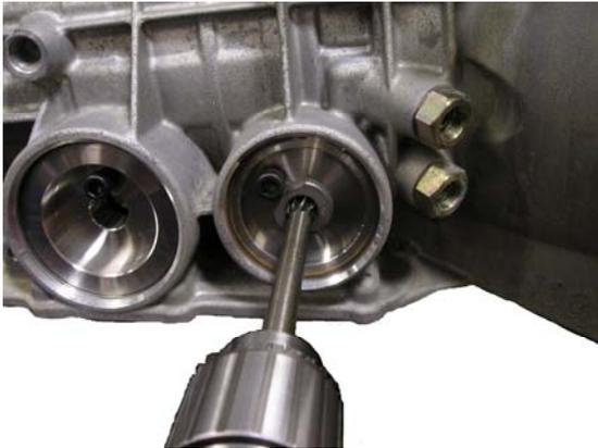
2. Drop the 9/16" guide into the jig. It doesn't matter which one of the lands on the guide you use, as long as one of the lands is under the 3/8" Allen screw.
